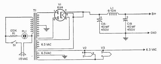
The schematic diagram for the oscillator and audio amplifier stages appears at the bottom of page 50. Unit is powered by full-wave rectifier and filament supply diagrammed above.
