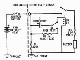
Small in size, the Belt-Minder packs a powerful buzzer in its all-aluminum case. Testing is simple—just depress push-button switch on bottom of unit for one second, then release. Buzzer should come on.
