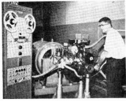
Road test simulating in the labs allows the engineers to compare various engine designs and parts under identical test conditions.
