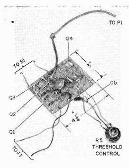
Almost all of the parts are mounted on a 3-by-41/4-inch phenolic circuit board. Use stranded wire for leads leaving the board.
