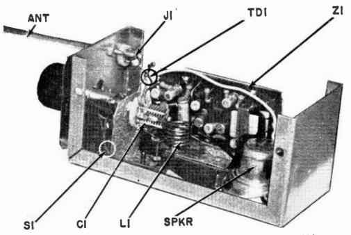
It's a tight fit inside the aluminum  $2\frac{1}{4}$ "  $\times$   $2\frac{1}{4}$ "  $\times$  5" chassis box. It would be best to copy the author's original layout of parts to avoid construction problems.
