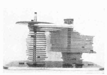
Plastic disks cut to scale (1 inch equals 20 feet) are stacked one on top of the other to give well makers an exact model of the underground cavern washed from the salt bed. Irregular shape results from different solubility of varying strata of the salt beds. Model at left shows a very deep well. Model above shows how two caverns were accidentally connected together by a washout that only the sonar caliper can discover.
