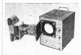
Quick-print Polaroid camera records oscilloscope pattern at each elevation measured.
