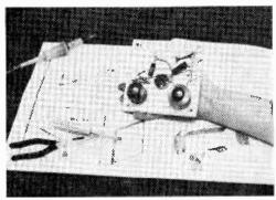
Crossover network wiring is simplified by pasting same-size pictorial on the board.
