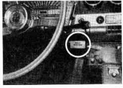
Installed out-of-the-way under the dash board, unit has only one wire connection. Be sure that hardware securing the auto belt minder provides a good ground between the aluminum box and the metal dashboard.
