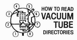
elements, but only five are brought out separately to the pin connections. They include the heater, cathode, control grid, screen grid and plate. The suppressor grid is connected internally to the cathode and is not counted as a separate active element.
