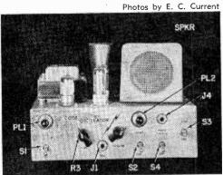
Sight & Sound code practice oscillator is all set to go. Just plug in telegraph key. Front panel decals give unit a professional touch.
