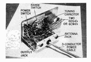
The Ameco Model PCL pre-amplifier packs a lot of electronics in its 3" x 5" x 3" case. Priced at \$24.95, the PCL can be tabbed a bargain booster.
