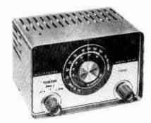
unit from line voltage variations. Illuminated plexiglass dial is calibrated from 50-54 mc. (6 meters) and 114-148 mc. (2 meters). Output voltage is 10-20 volts rms. Priced at \$29.95, the HE-89 operates on 115-volt 50/60 cps power. (Lafayette Radio Electronics Corporation, 111 Jericho Turnpike, Syosset, L. I., New York)
