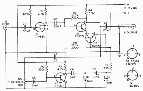
The unusual symbol for Q1 indicates the part is a field effect transistor. Its case resembles Q1's and Q2's. Part placement is not critical, however, try to duplicate the original design.
