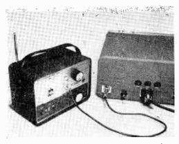
Here, the Ten-2 CB Checker is connected to the antenna terminal of the CB rig under test. One tester can rate your CB gear.
