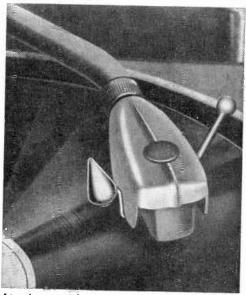
Atomic particles radiating from a small Audiotex 30-002 emitter clipped to tone arm kills static charges from disc surface.
