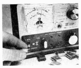
One function of the Ten-2 is checking activity of CB crystals. Both standard and handie-talkie types can be tested.
