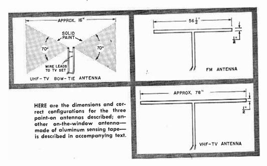
13) and for FM frequencies, a folded dipole configuration is best. UHF-TV takes a different type, described later.
