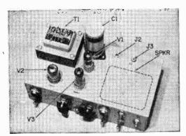
Placement of parts is not critical. A large aluminum chassis provides ample room for the control panel parts and neat layout, too.
