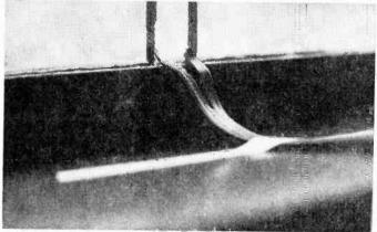
ENDS of twin lead from TV are stripped of insulation, then fanned out and laid against base of painted conductors where they are bonded with liberal dabs of conductive silver paint.
