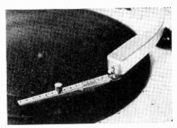
Stylus pressure gauge helps make correct tone arm tracking pressure adjustment. This adjustment prevents rapid record and stylus wear due to excessive pressure.
