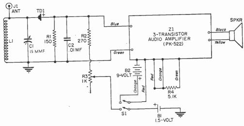
The placement of parts in the RF section is critical, but neatness in construction will lick more than half the problem. Keep leads and parts away from coil L1 and capacitor C1.
