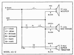
Schematic diagram of the crossover network. The speaker system's impedance is 8 ohms.
