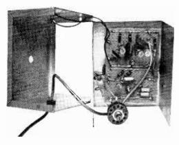
The CB-Lim prior to final assembly. There is enough room inside to mount dry cells.
